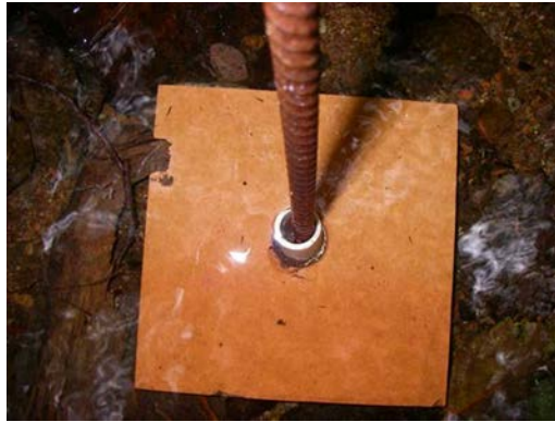
Figure 13-2. Unglazed ceramic tile (approximately 15 × 15 cm) anchored to stream bed with rebar.
