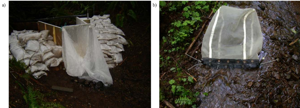
Figure 12-3. Drift net deployment in the Type N Study sites with a flume (a) and without a flume (b).
