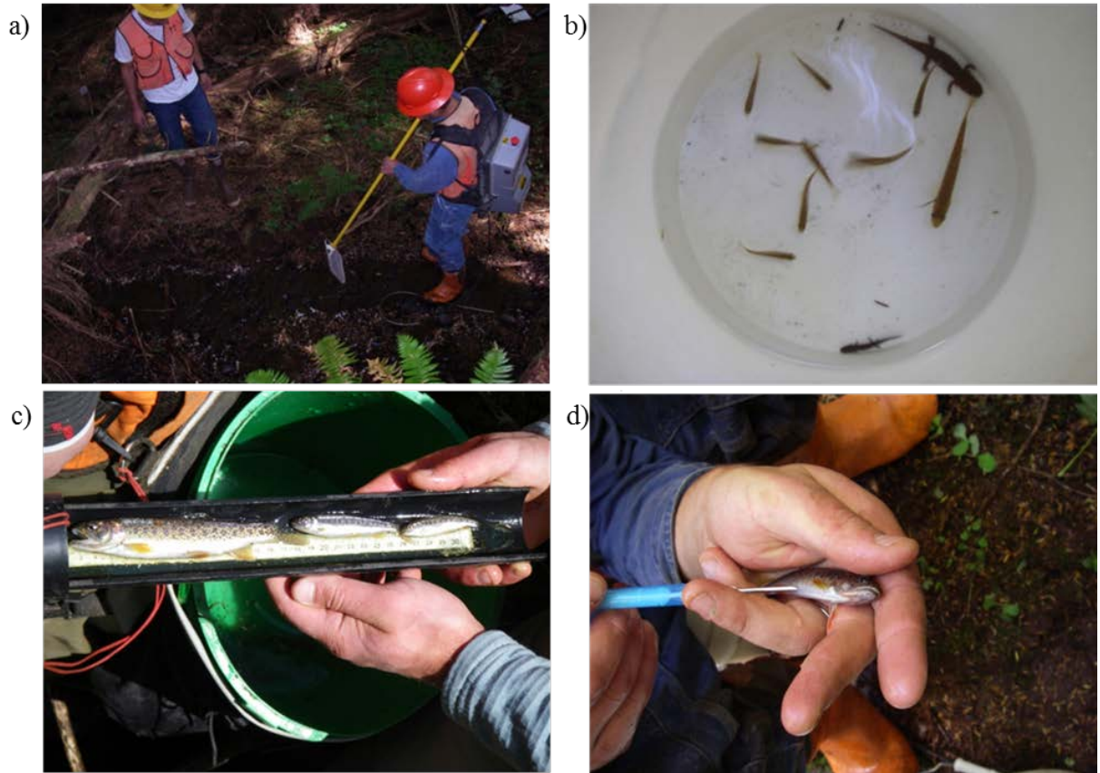
Figure 16-2. Conducting fish surveys for the Type N Study: (a) electrofishing a typical Type N study reach; (b) typical catch from a single electrofishing pass through a Type N study reach (note 5-gallon bucket for scale); (c) representative coastal cutthroat trout from three different cohorts on length board for scale; and (d) PIT tagging of a coastal cutthroat trout.
