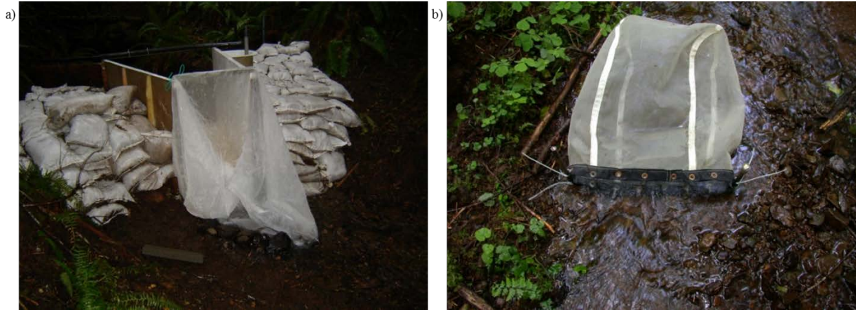
Figure 14-5. Drift net deployment in the Type N Study sites with a flume (a) and without a flume (b).
