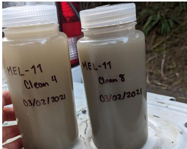
Figure 5.3 Wash-off samples collected before (Clean 4) and after (Clean 8) multiple pickup truck passes over a 1'x1' area. The change in clarity of the samples demonstrates an increase in fine sediment post truck pass.
