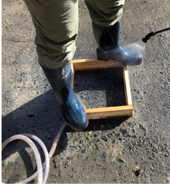
Figure 5.2 The fine sediment that is available for transport on the road surface due to recent traffic is carefully washed from the isolated sampling area and evacuated into a sample container for sediment analysis.
