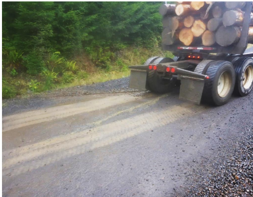
Figure 5.1 New fine sediment pumped from the roadbed by the passage of a loaded log truck.
