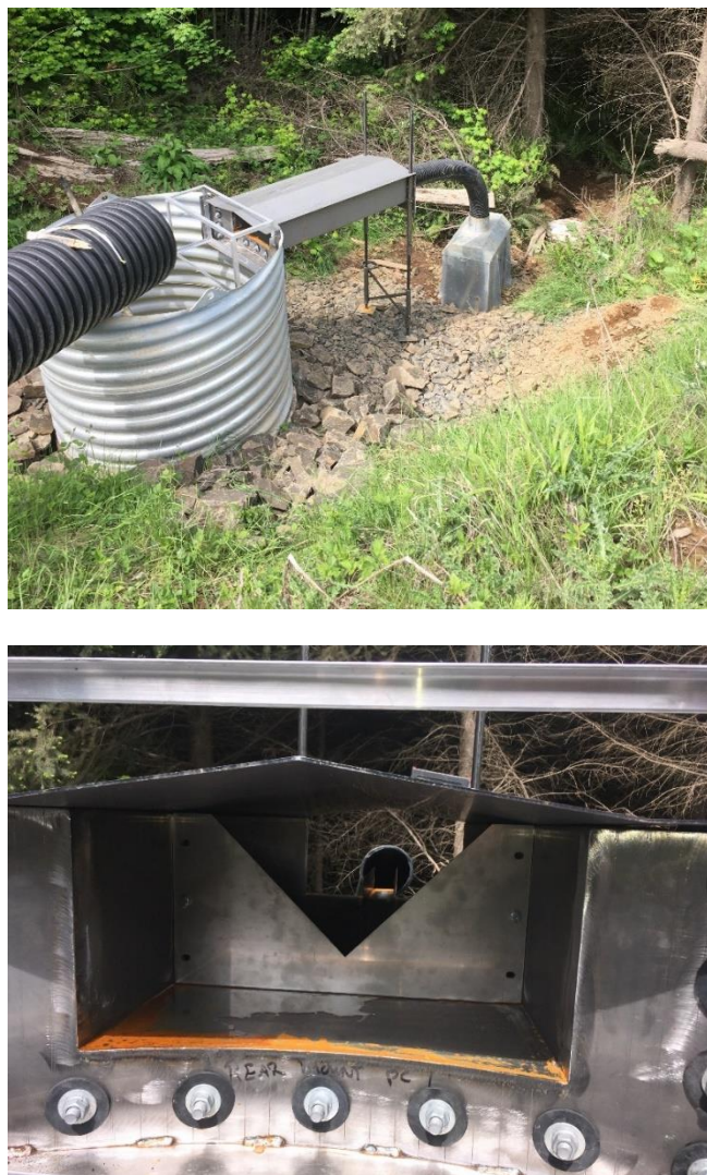
Figure 1.5 V-notch weir and flow-proportional splitter prototype in upper photo. View from inside the tub along the water flow path in lower photo.
