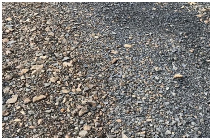
Figure 1.2 “Good” rock (i.e., relatively unweathered basalt) is the darker rock in this picture, and “marginal” rock (i.e., slightly more weathered) appears with a lighter tan color. Good rock is used at most sites in practice, and marginal rock has been applied at approximately one-half of the sites to test the effects of rock quality on sediment yield.
