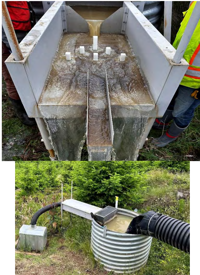
Figure 3.5 V-notch weir and flow-proportional splitter in upper photo. The white blocks spread the water to ensure even flow across the splitter at the end of the flume. The lower photo shows the covered flume, debris filter and the stage measuring sensor in the white tube. The black material at the end of the culvert is a flow diffuser that prevents water from overtopping the tub at high flows.
