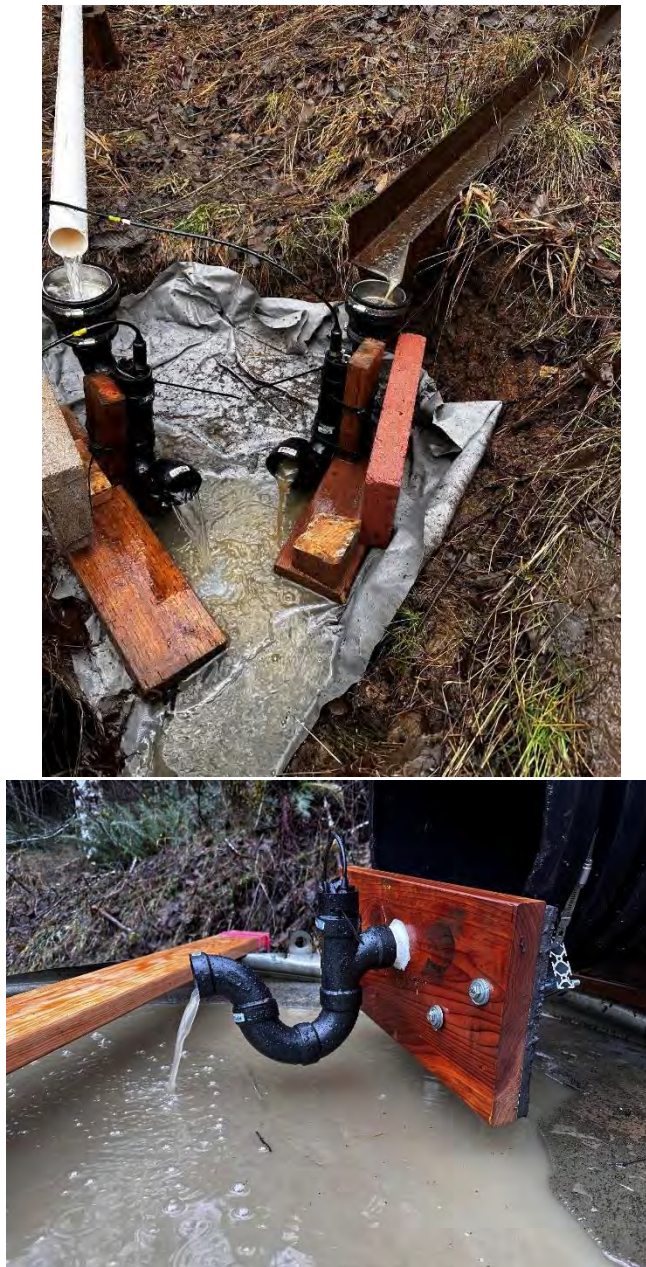
Figure 6.9 Turbidity sampling locations below the trough and ditch in the upper photo and at the Tub in the lower photo.
