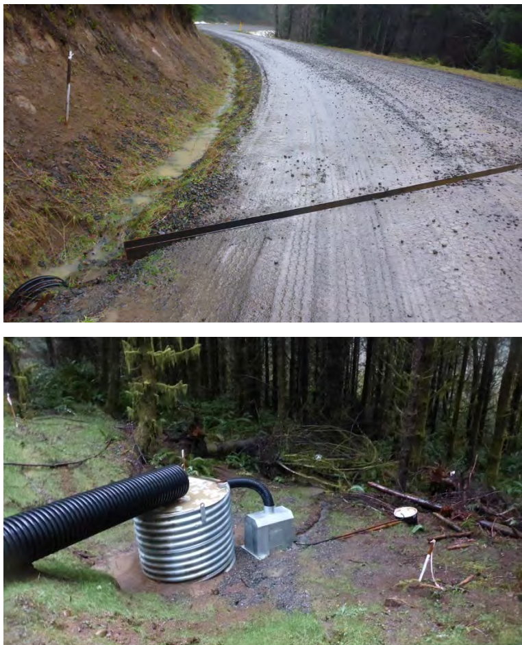
Figure 3.4 The upper figure shows the road surface routing water to the ditch and the collection trough. Water and sediment then are routed through a culvert pipe to the sediment tub. The lower figure shows the platform with the sediment tub collecting road sediment, the tipping bucket measuring discharge and the suspended sediment tank (SST) sampling the fine sediment that is not settled in the tub.
