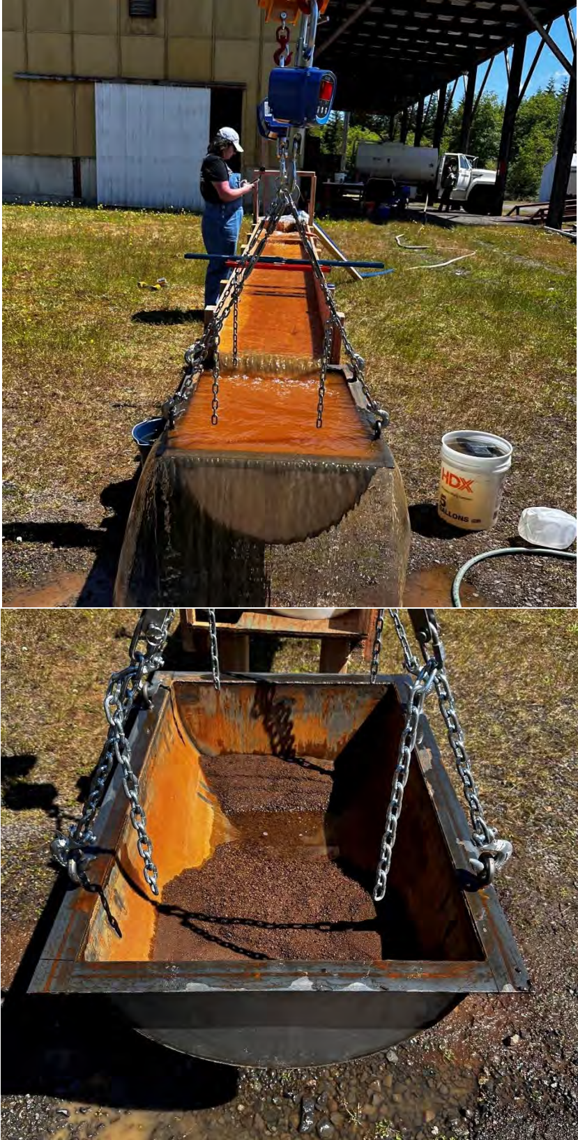
Figure 5.2 Flume with sampler during run in the upper image and the retained sample in the photo below.
