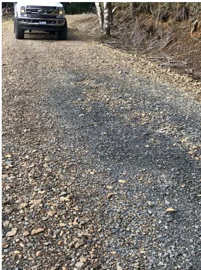
Figure 3.2 “Good” rock (i.e., relatively un-weathered basalt) is the darker rock in this picture, and “marginal” rock (i.e., slightly more weathered) appears with a lighter tan color. Good rock is used at most sites in practice, and marginal rock has been applied at half of the sites to test the effects of rock quality on sediment yield.
