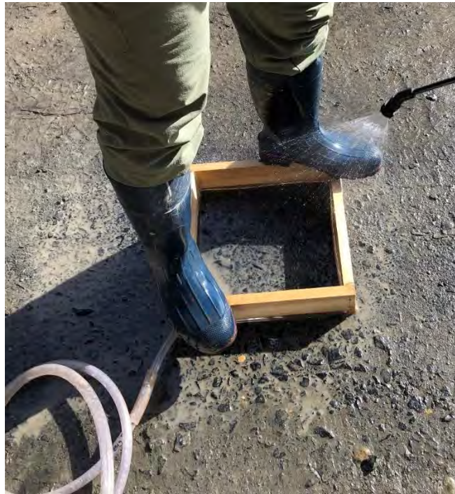
Figure 6.3 The fine sediment that is available for transport on the road surface due to recent traffic is carefully washed from the isolated sampling area and evacuated into a sample container for sediment analysis.
