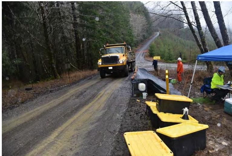
Figure 6.8 Gutter is sheltered from direct rainfall with a cover so that the sample is not diluted.
