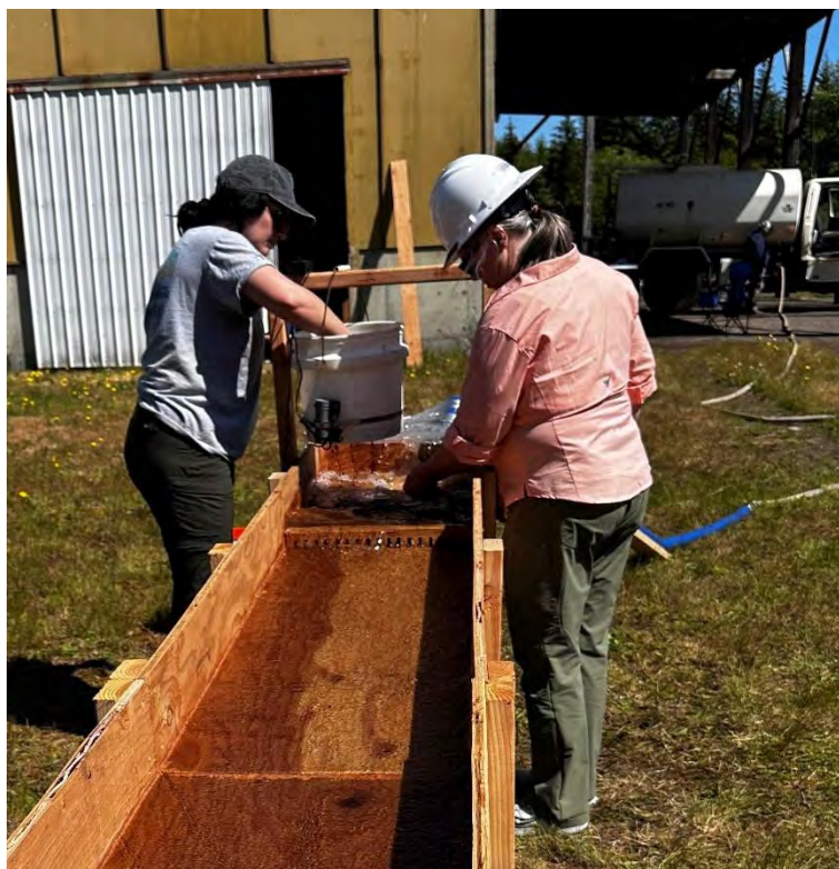
Figure 5.3 Vibratory sediment feed device applying the sediment at the upper end of the flume.
